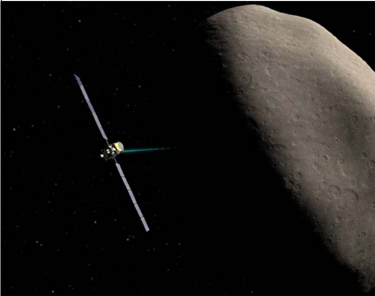
Dawn will be the first spacecraft to establish orbits around two separate target bodies during its mission—thanks to ion propulsion validated by Deep Space 1. Image by: NASA
