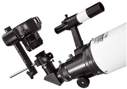
Fig. 1 This adapter allows to connect virtually any point-and-shoot camera to a telescope for eyepiece projection photography.
