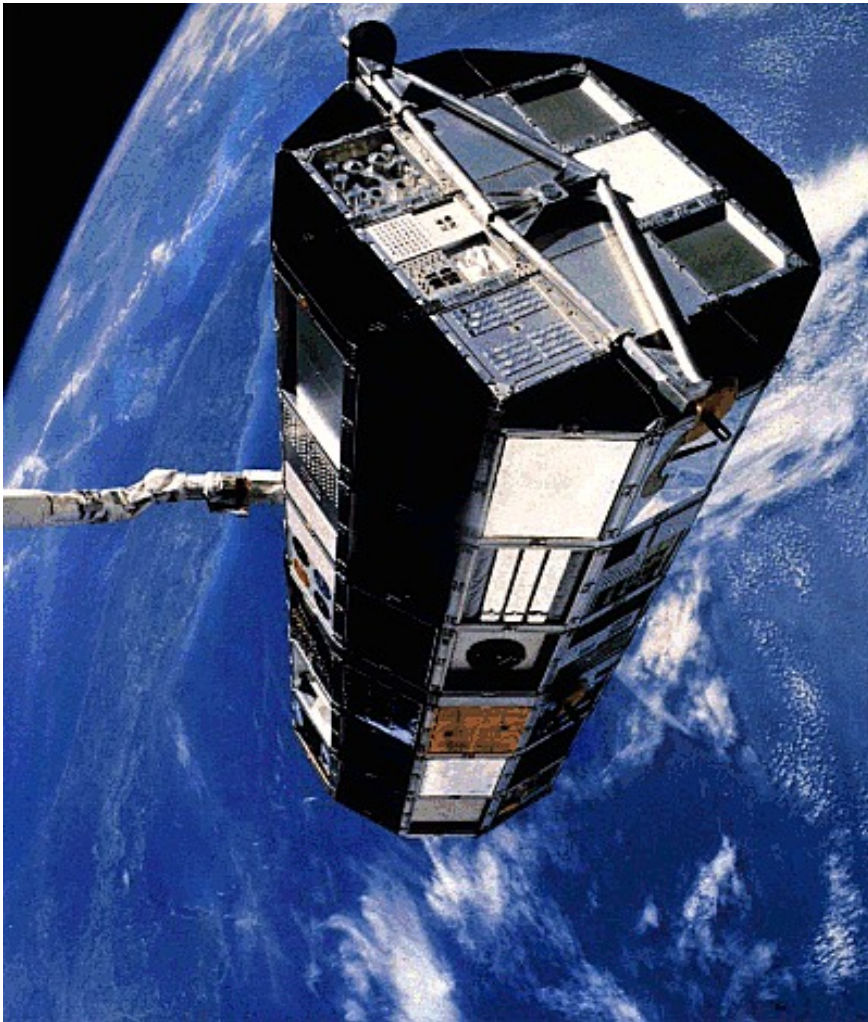
Fig. 4. LDEF. JPO was a co-investigator and member of the science team that analyzed data collected by the Long Duration Exposure Facility spacecraft. Launched in 1984, LDEF remained in orbit for almost 6 years. Precise times of impacts were recorded for the first 346 days in orbit. (Cred. NASA Langley Research Center.)
